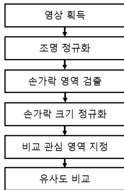
Fig. 1. Procedure of Proposed Thumb Recognition Method
