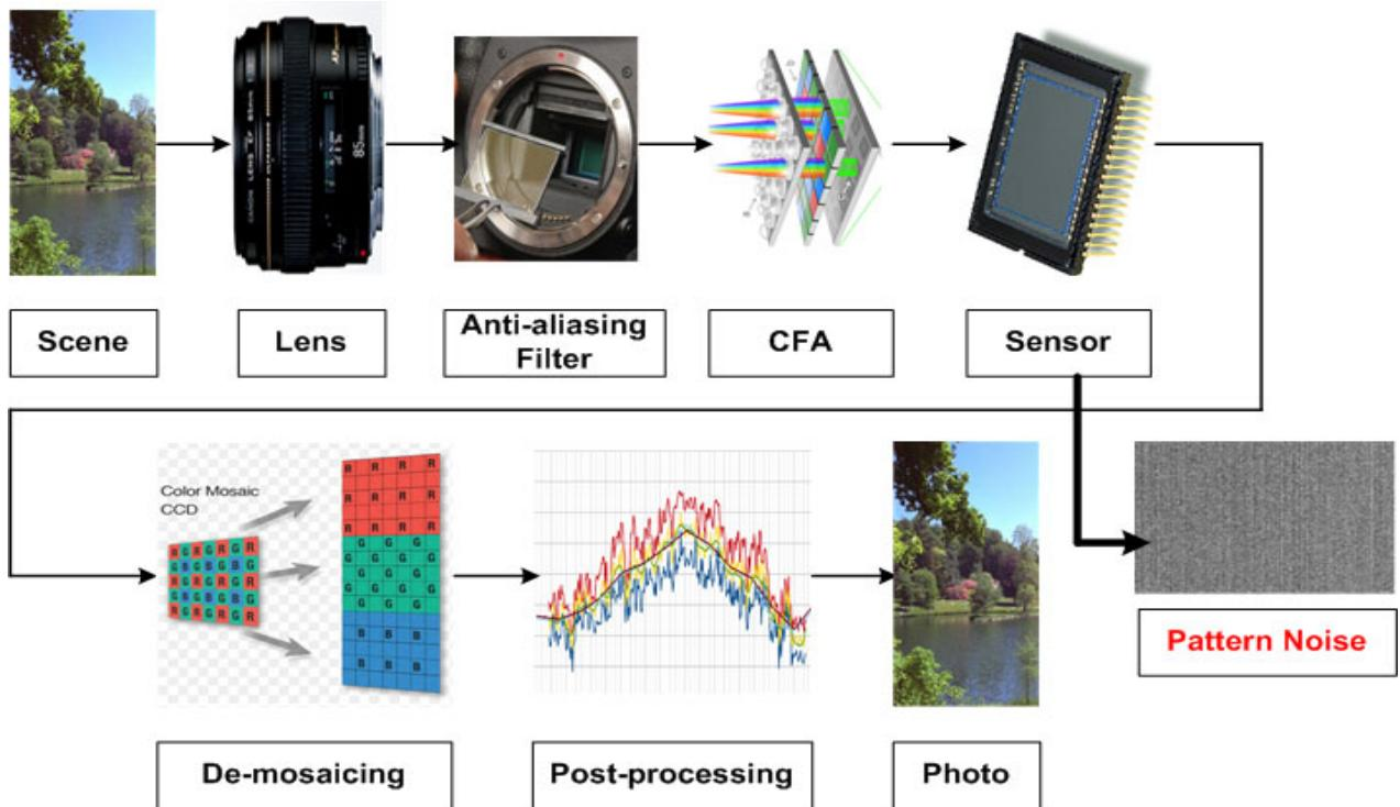
Fig. 1. Image Acquisition Process in Digital Imaging Devices
