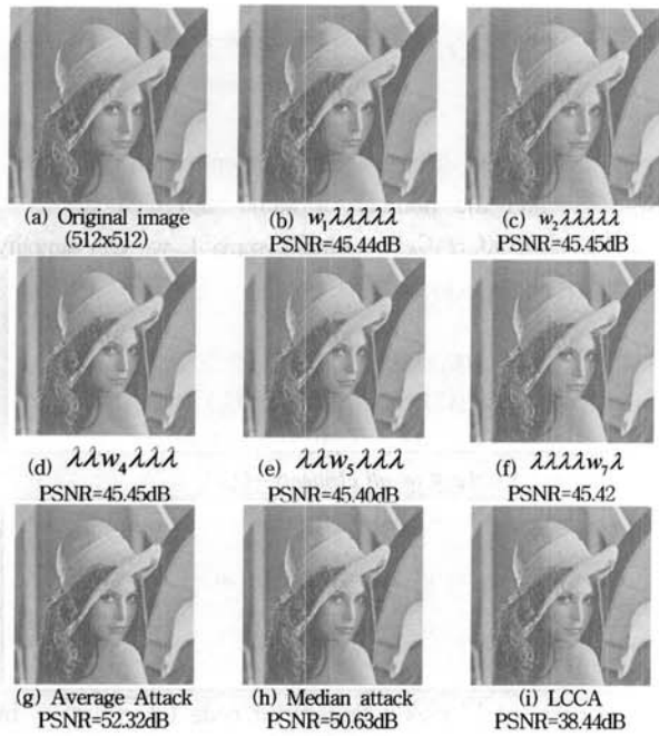
(Fig. 3) (a) Original, (b-f) five colluders' fingerprinted images, and colluded images after (g) average attack, (h) median attack, (i) LCCA
