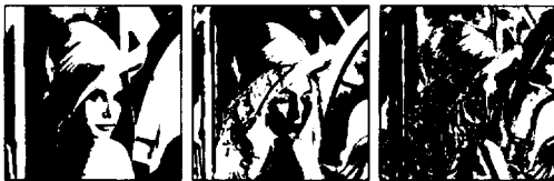
(a) b_7 bit-plane image (c) b_5 bit-plane image (b) b_6 bit-plane image
