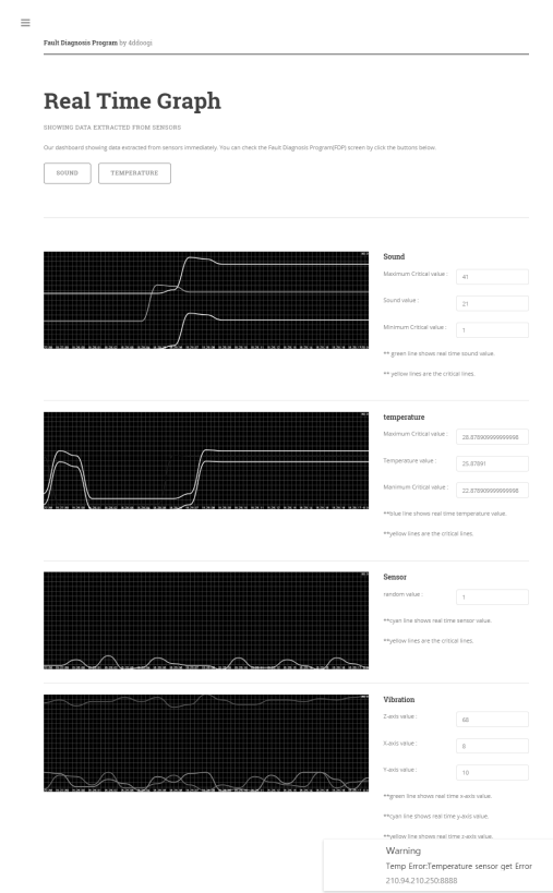
Fig. 3. Web Dashboard Displaying Sensor Information, Sensor Data from Multiple Sensors are Displayed Together to Show Current Environment's Status, Right Side Panel is used for Device Setting
