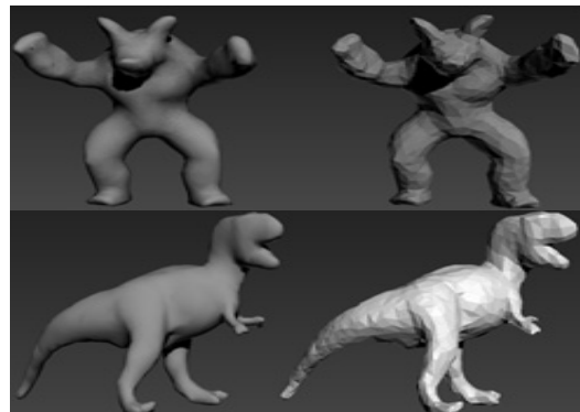
Fig. 2. The Result of the Conversion from a Surface Model to a Tetrahedral Model by Tetgen (left) Surface Model (right) Tetrahedral Model
