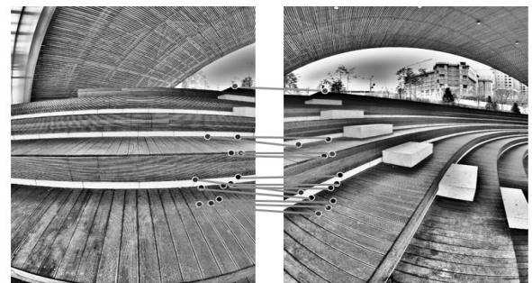
Fig. 8. Matching Relation of Corresponding Points after Applying RANSAC Algorithm
