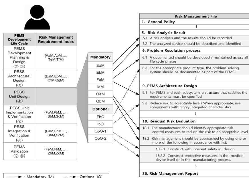
Fig. 4. Analysis process of Risk Management Items based on PEMS Development Life Cycle
