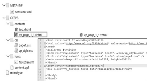
Fig. 4. 'Hello World' Representation Structure in EPUB 3.0
