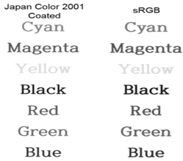
Fig. 9. Text Conversion using ICC Profiles
