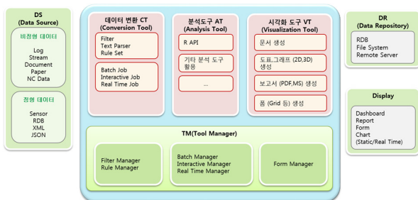
Fig 7. Structure of the Data Conversion, Analysis, and Visualization Tools
