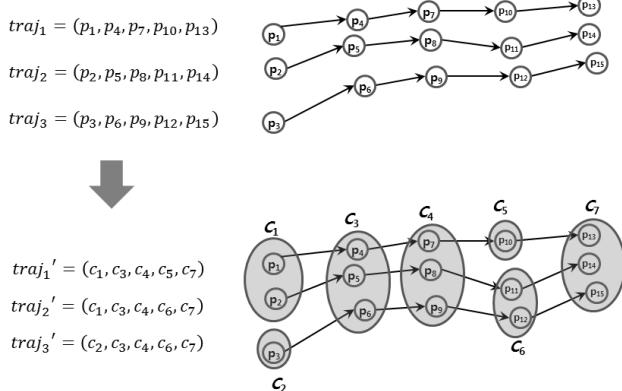
Fig. 2. Transformation of trajectories into POI sequences
