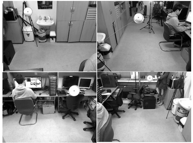
Fig. 5. Extracted calibration object in four RGB images
