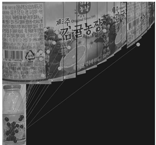
Fig. 12. The result of matching panorama model space and input image
