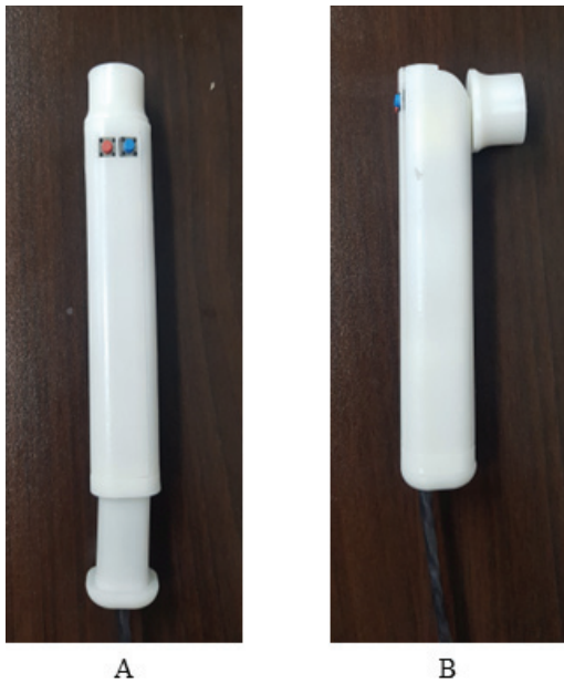
Fig. 4. MHC morphing states. A is the state of increasing the length of the MHC. B is a bending state of the MHC.
