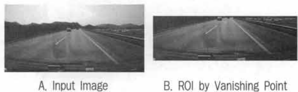
Fig. 7. ROI based on Vanishing Point
