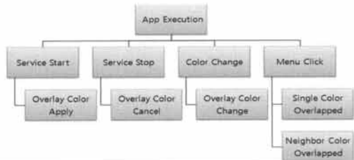
Fig. 4. Functional configuration of virtual overlays App
