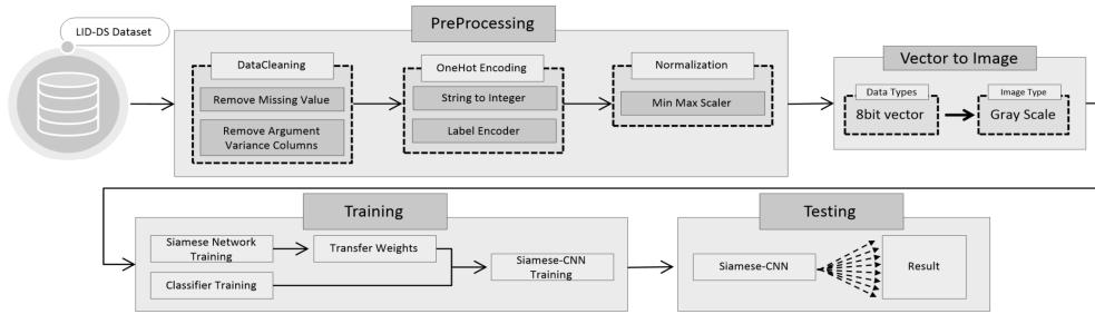
Fig. 1. Proposed Host-based Intrusion Detection Model Structure
