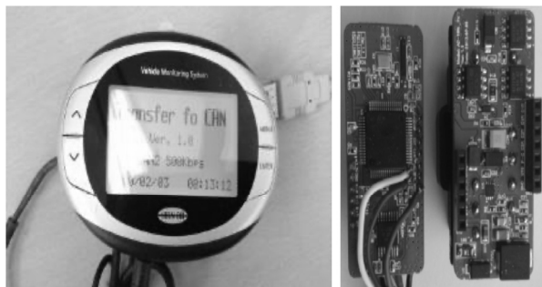
Fig. 3. OBDDI Device Display and PCB Hardware
