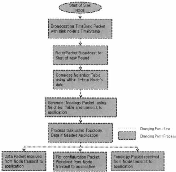
(Fig. 3) Step of Sink Node's processing
